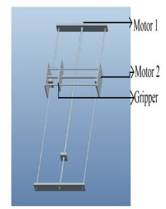
Fig. 2 CAD model of XY Table
