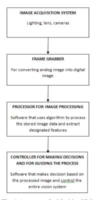
Fig. 1 Anatomy of a Machine Vision System
