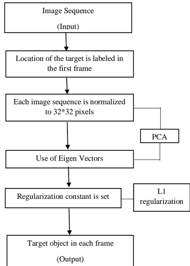
Fig. 2. Architecture of the tracking algorithm
