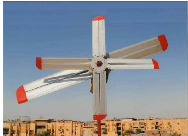
Figure (2), Counter Rotating Open Rotor
