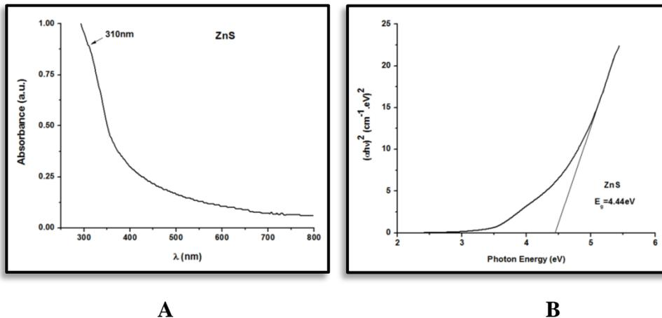
**Figure 9 A) UV-Vis absorption spectra of ZnS QDs, B) Tauc plot of ZnS QDs.**
