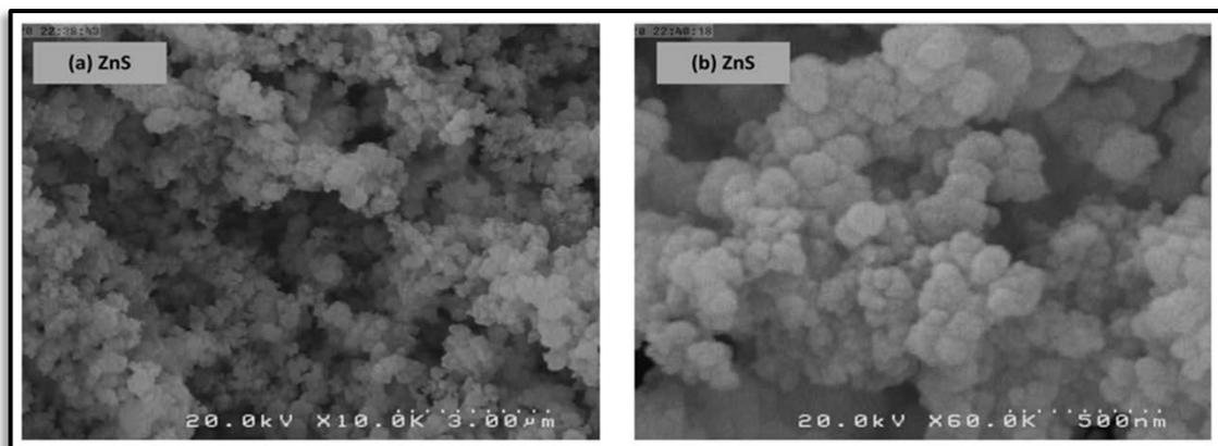
**Fig. 4 FESEM images of ZnS QDs (a) low magnification, (b) high magnification.**
