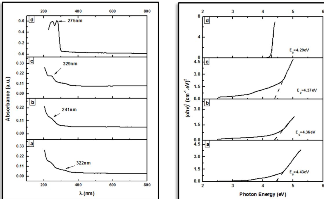
**Figure 10 (A) UV-Vis absorption spectra of Mn doped ZnS QDs, (B) Tauc plot; (a,b,c & d are corresponding to doping concentrations 1%, 2%, 3% and 4%) respectively.**
