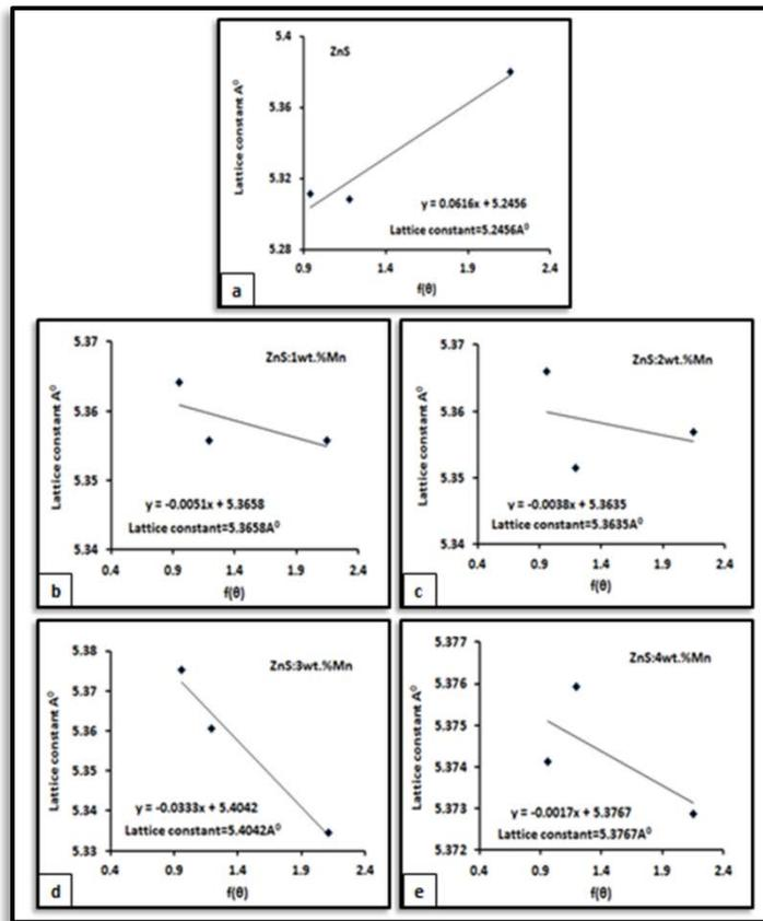
**Fig. 2 Nelson-Riley plot of nanocrystalline Mn doped ZnS QDs; (a, b, c, d & e corresponding to (0, 1, 2, 3 & 4) wt.%Mn respectively).**
