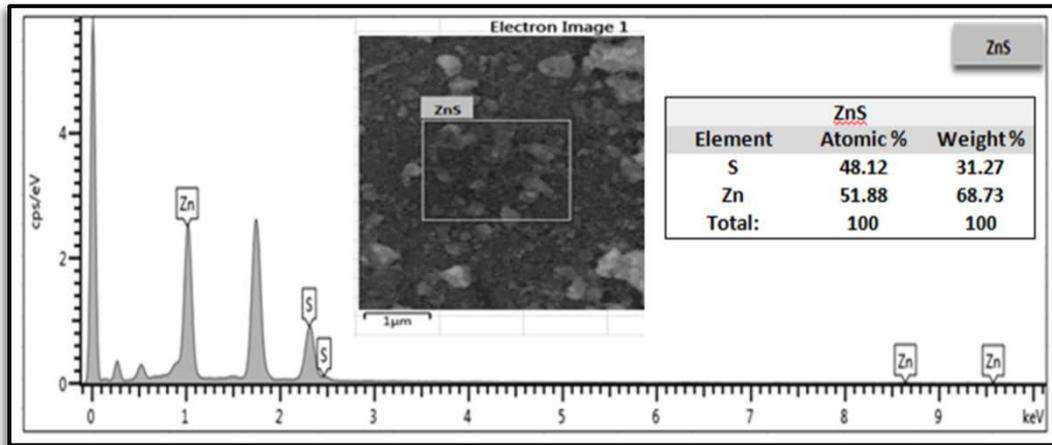
**Fig.7 EDS spectrum for pure ZnS.**
