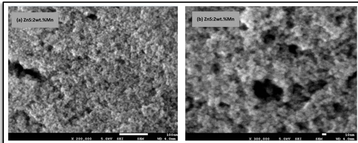
**Fig. 6 HR-FESEM images of Mn doped ZnS QDs (a) low magnification, (b) high magnification.**
