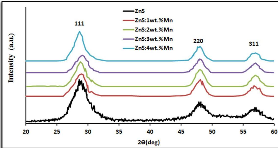
**Fig.1 XRD patterns for undoped and manganese doped ZnS.**
