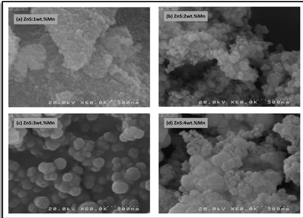
**Fig. 5 FESEM images of Mn doped ZnS QDs; (a,b,c & d are corresponding to doping concentrations 1%, 2%, 3% and 4%) respectively.**
