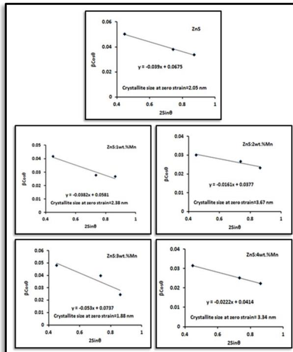
**Fig. 3 Stokes-Wilson plot of nanocrystalline undoped and doped ZnS QDs.**
