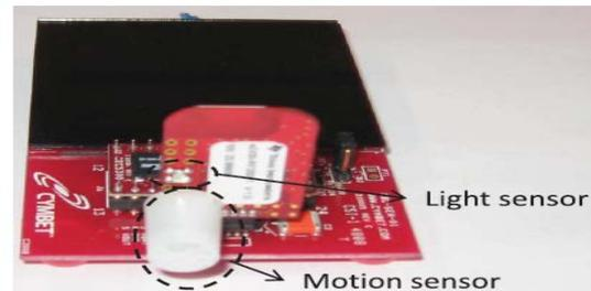
Fig.5: Light harvesting wireless sensor module
