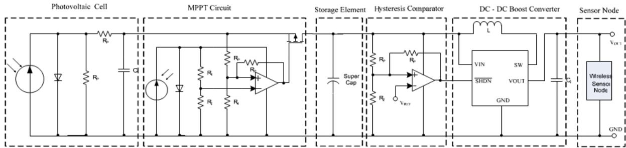
Fig.1: The block diagram of the proposed power management system.
