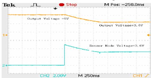
Fig.3: Measured waveform of Output voltage and the wireless sensor node voltage while transmitting signal load.
