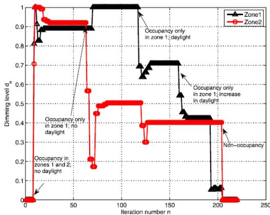
Fig.7: Dimming levels of luminaires in the two zones over control iterations with dynamic occupancy and daylight.
