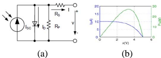
Fig.2: (a) Electrical model of PV cell
