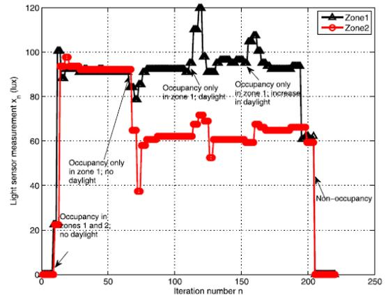
Fig.8: Light sensor measurement in the two zones over control iterations with dynamic occupancy and daylight.
