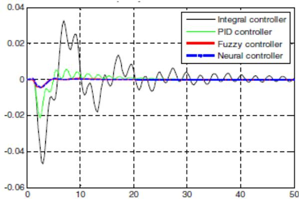
Fig. 8 Frequency deviation of area-2
