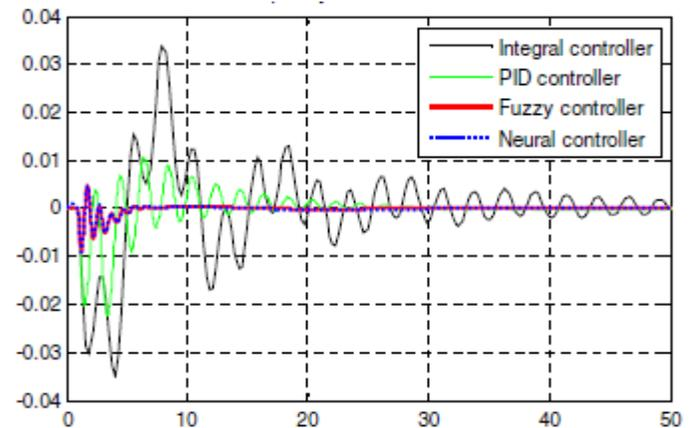
Fig. 7 Frequency deviation of area
