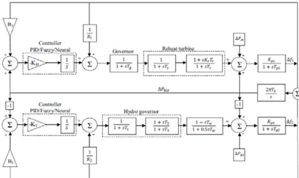
Figure.1. Two area Hydro-Thermal power system
