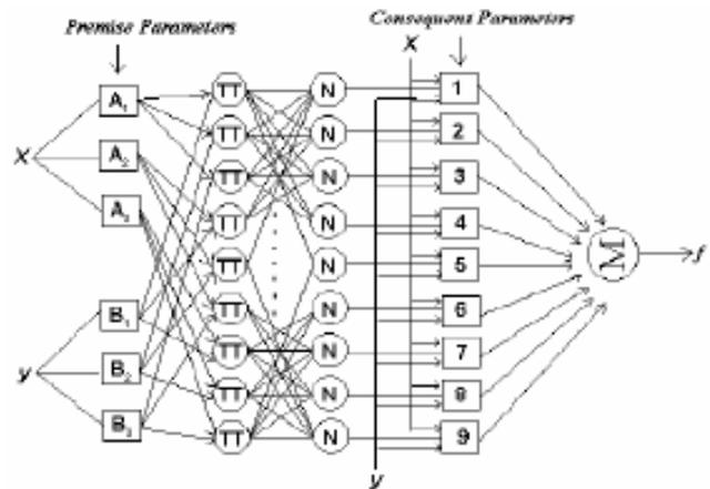
Fig. 2 Architecture of a Two-Input Sugeno Fuzzy Model with Nine Rules
