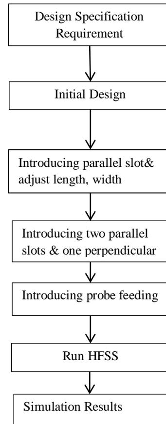
Fig.2 Antenna Design Procedure
