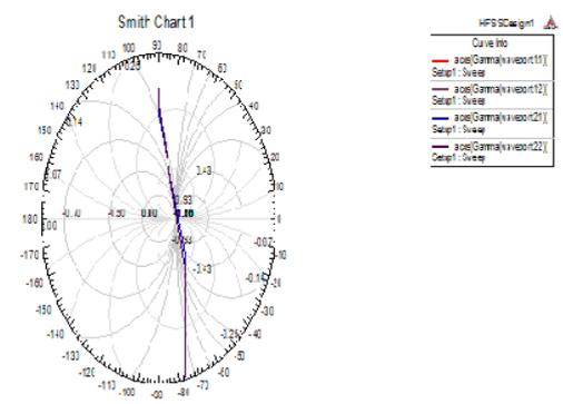
Fig.7 Performance of antenna using Smith chart
