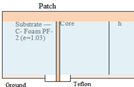
Fig.4 Cut Plane View of Antenna
