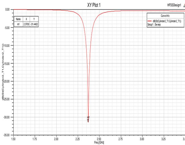
Fig.9 S-Parameter of optimized antenna
