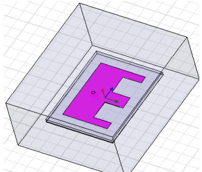
Fig.1 Proposed E-Shaped Patch Antenna
