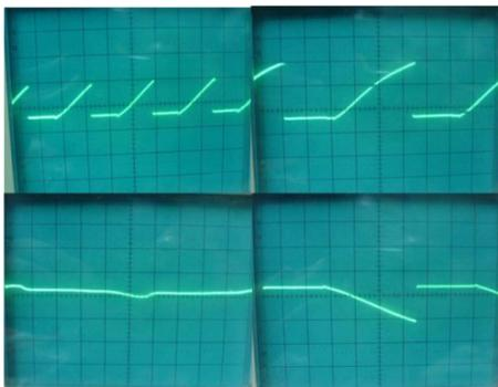
Figure: PWM duty cycle motor control output.
