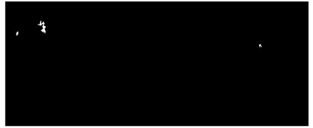
Fig.9. Flaws having intensity above high threshold value
