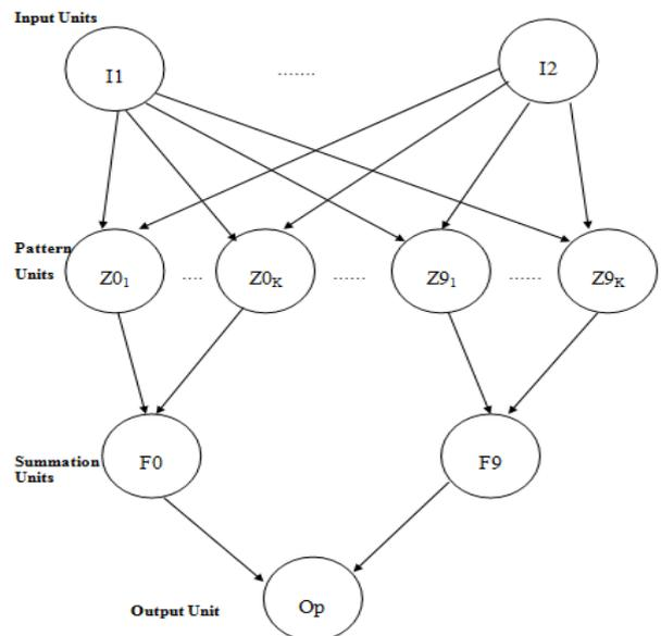
Fig. 2 Architecture of Probabilistic Neural Net
