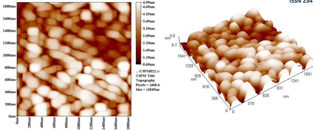
**Fig. (2):** 2D and 3D views of AFM image of  $\text{Al}_2\text{O}_3$  nanoparticles applied on pure Al.
