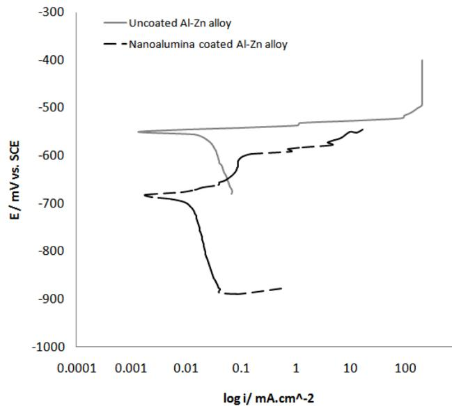
**Fig. (8):** Potentiodynamic polarization for uncoated and nanocoated Al-Zn alloy in seawater.
