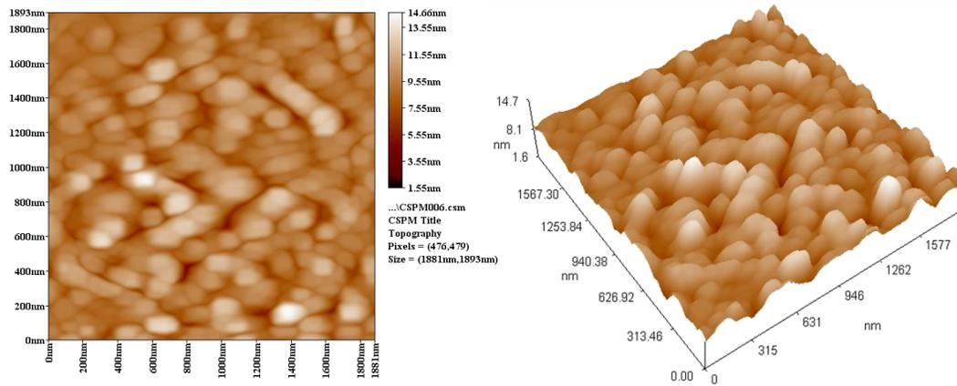
**Fig. (3):** 2D and 3D views of AFM image of  $\text{Al}_2\text{O}_3$  nanoparticles applied on Al-Si alloy.
