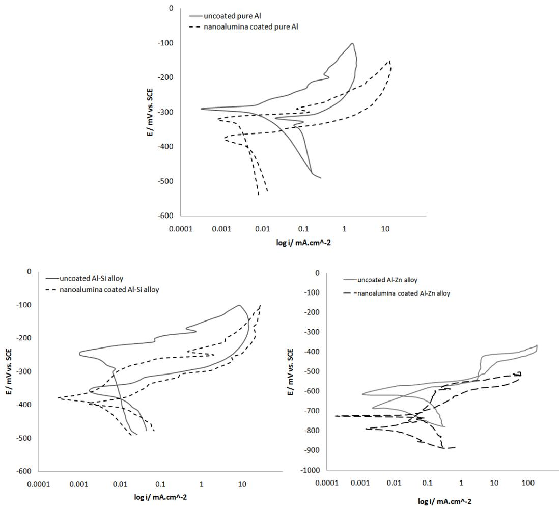
**Fig. (9):** Cyclic polarization for uncoated and nanocoated pure Al and its alloys in seawater.
