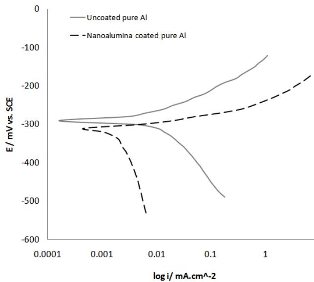
**Fig. (6):** Potentiodynamic polarization for uncoated and nanoaluminum coated pure Al in seawater.
