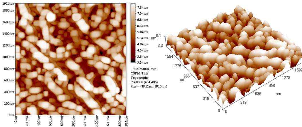
**Fig. (4):** 2D and 3D views of AFM image of  $\text{Al}_2\text{O}_3$  nanoparticles applied on Al-Zn alloy
