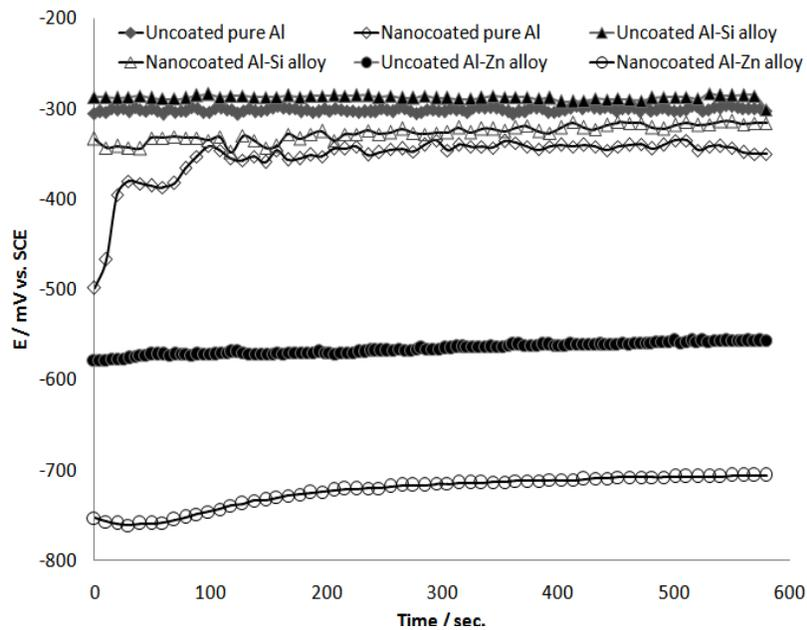
**Fig. (5):** The variation of potential versus time for uncoated and nanocoated pure Al and its alloys in 3.5% M NaCl solution at room temperature.
