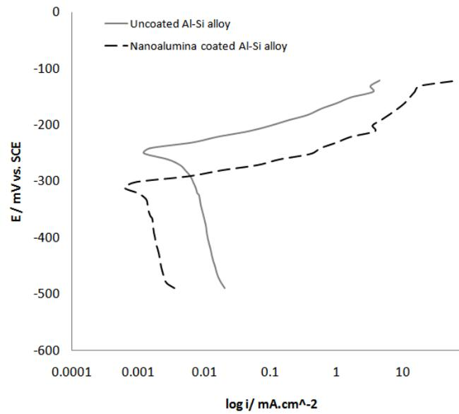
**Fig. (7):** Potentiodynamic polarization for uncoated and nanocoated Al-Si alloy in seawater.
