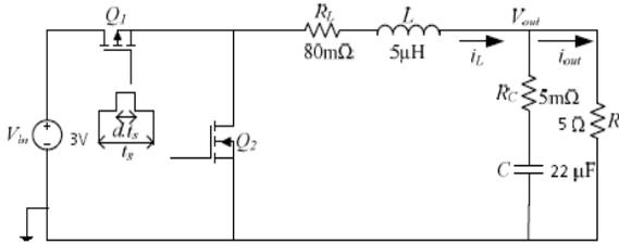
Fig. 1 Buck converter circuit model
