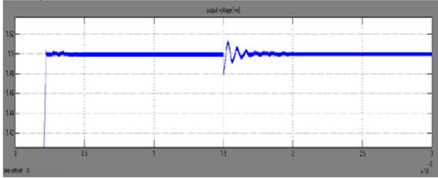
Fig. 9 Output Voltage Response for Change in Load
