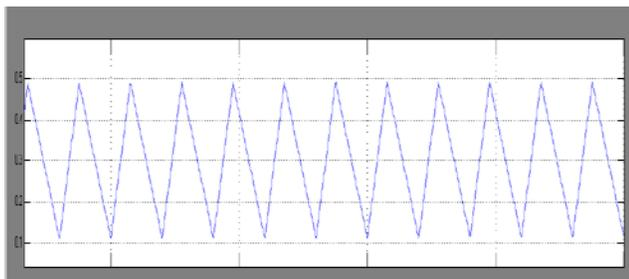
Fig. 12 Inductor Current Ripple for Change in Supply
