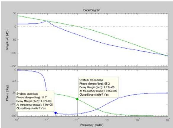
Fig 4 Bode Plot of the Closed Loop and Open Loop Converter.
