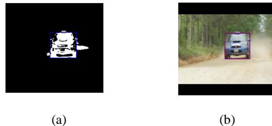
Fig. 4 Implementation of track the invariant feature. (a) Window across interested region in Blue color. (b) Track that window using kalman filter in red color.
