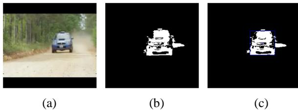
Fig. 2 Implementation of feature descriptor a) Original frame b) Detect interest point using BS with color c) Plot the window across interested region in blue color.
