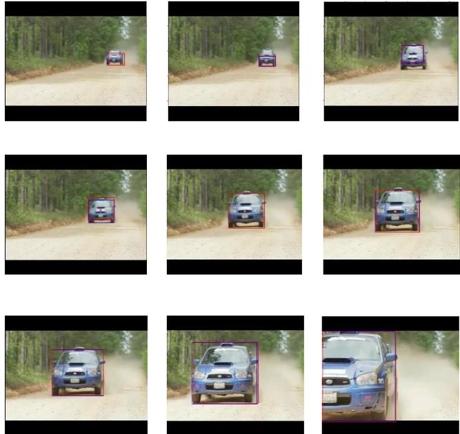
This experiment result using invariant feature tracking and color tracking with kalman filter to track an object in MATLAB on the computer AMD dual-core 1.333 Ghz Aspire one 725 and video frame size is 320\*240.
