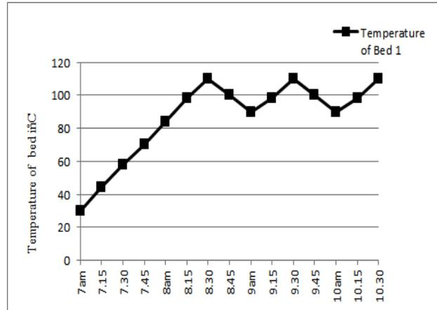
Fig3. The Maintained Temperature in Adsorbent Bed 1
