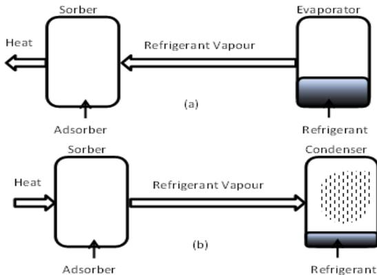
Fig. 1 (a) Adsorption (Refrigeration) Process
