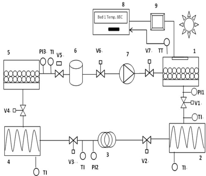
Fig. 2 Experimental setup of An Energy Efficient Air Conditioner System without Compressor: Application of Embedded Systems. (1- Adsorbent Bed1, 2-Condenser, 3-Expansion valve, 4-Evaporator, 5- Adsorbent Bed2, 6-Reservoir, 7-12 VDC Pump, 8-Microcontroller, 9- Power Control Device, PI- Pressure Indicator, TI-Temperature Indicator, TT-Temperature Transmitter, V1-V7 Valves ) effect. The evaporator cools 10°C less than room temperature. This process is called adsorption or regeneration process.
