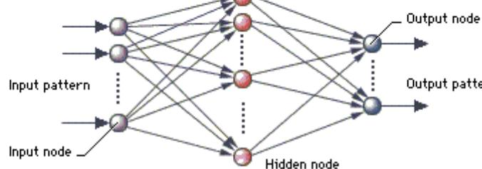
**Diagram 1: Basic Structure of Neural and artificial neural network [9]**
