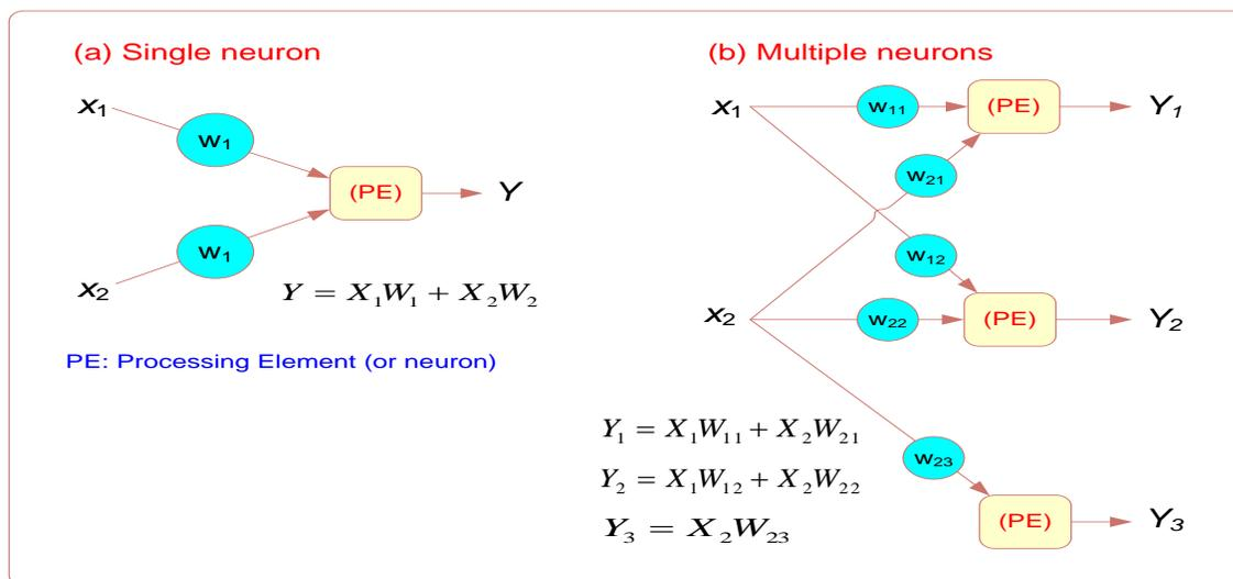
**Diagram 2: Structure of single Neuron and Multiple Neurons.**
