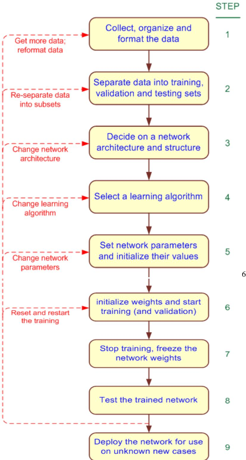
**Diagram 3: Development Process of an Artificial Neural network [2]**
