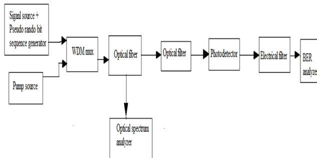
Fig.1: 10 Gb/s optical wavelength conversion set up
