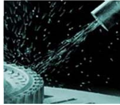
Fig: 2.1.2. Shot peening for longer fatigue life
