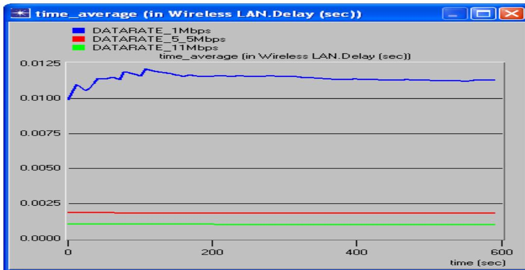
Fig 2: Delay Study for Data-rates of 1Mbps, 5.5Mbps and 11Mbps
