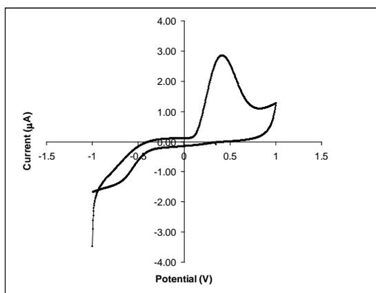
Fig. 3 Cyclic voltammogram for catechin (200 mg/L) using S2
