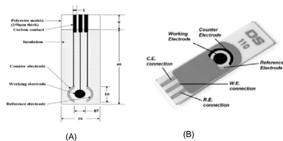
Fig. 1 Schematic representation of S1 transducer (all dimensions are in mm) (A) and S2 transducer (B)
