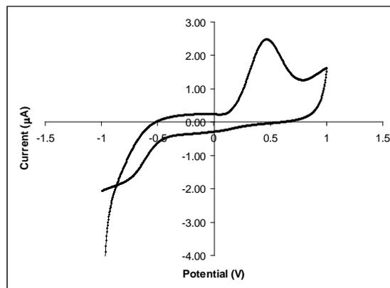
Fig. 2 Cyclic voltammogram for catechin (200 mg/L) using S1
