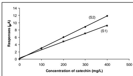
Fig. 4 Comparison between calibration curves for catechin using different electrodes (S1 and S2): (S1)  $y = 0.0225x + 0.2959$ ;  $R^2 = 0.9954$ ; (S2)  $y = 0.0295x + 0.057$ ;  $R^2 = 0.9998$
