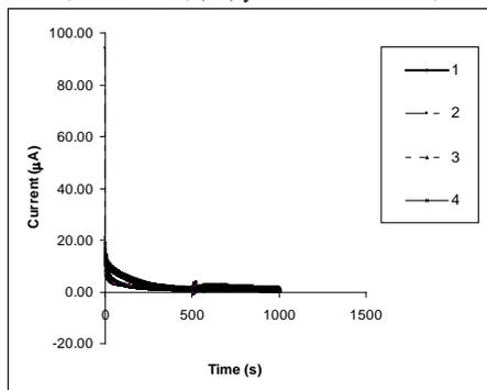
Fig. 5 Effect of presence of probable interfering substances on response given by screen printed electrode (S1). (1)Amino acid (D-phenylalanine), (2)Ascorbic acid (3)Carbohydrate (D-fructose) (4)Organic acid (oxalic acid)
