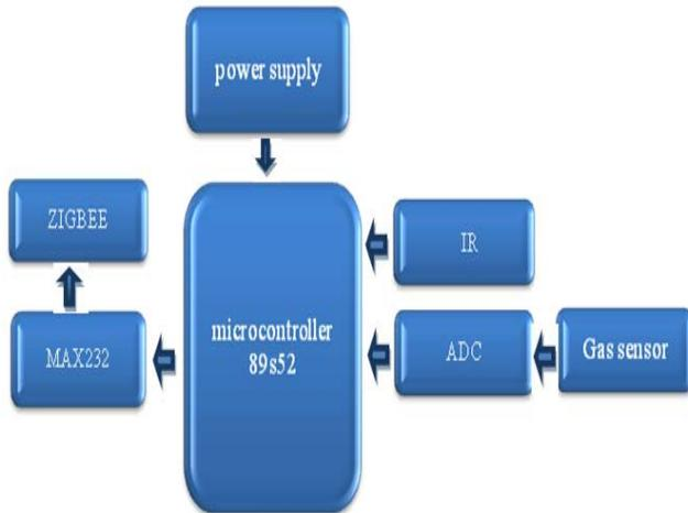
Fig. 1 Smart trash system
