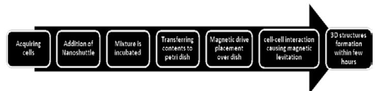
Fig 2: Block diagram for 3D Magnetic bio printing
