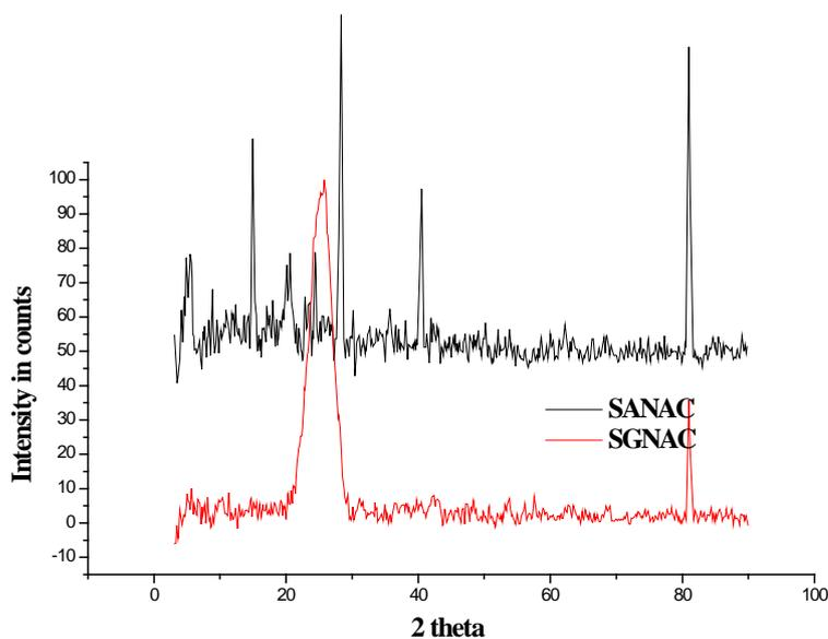
**Fig. 4 XRD pattern of SANAC and SGNAC after adsorption of chromium.**
