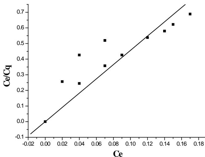
**Fig. 5. Langmuir isotherm for Cr (VI) adsorption.**
