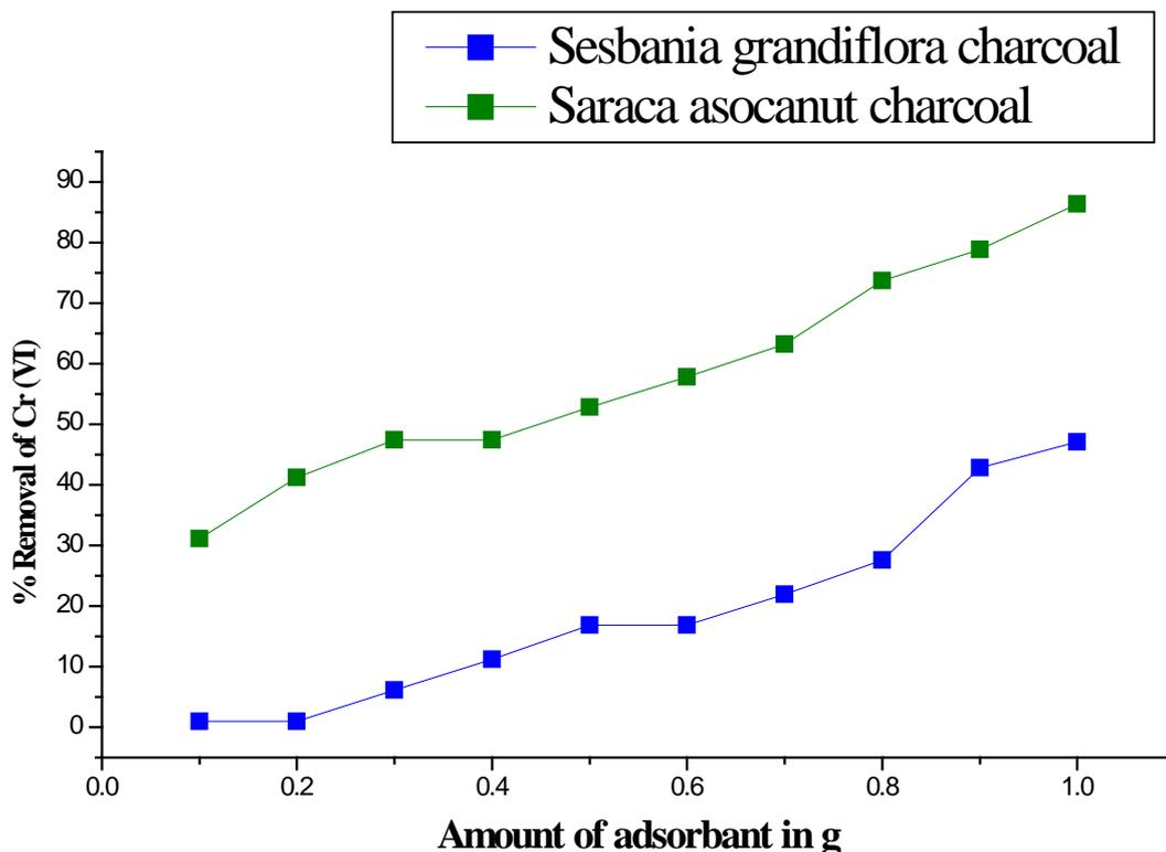
**Fig.2 Effect of adsorbate concentration on the SGNAC and SANAC.**
