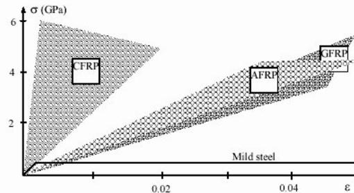
Fig. 2. Uniaxial tension stress-strain diagrams for different unidirectional FRPs and steel. CFRP = carbon FRP, AFRP = aramid FRP, GFRP = glass FRP [9].
