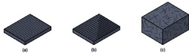
Fig 6. Fiber orientation in a) continuous b)woven and c) chopped form
