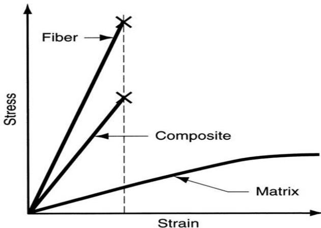
Fig 1. Stress Strain Diagram for Composite Phases
