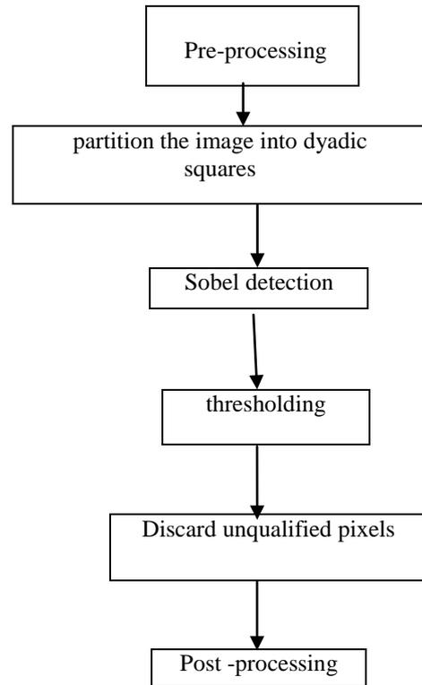
Fig.5 Proposed architecture by Xilinx system generator
