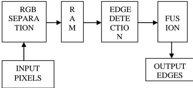
Fig 3 Proposed Architecture using Xilinx
