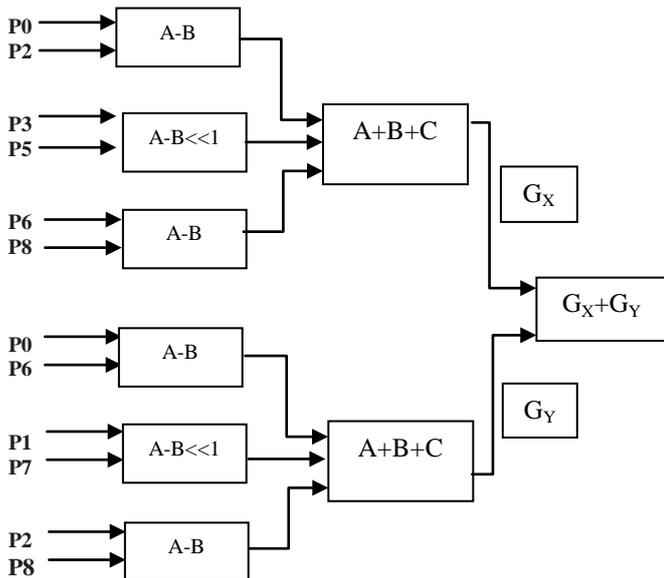
Fig.4 Modified gradient block diagram.
