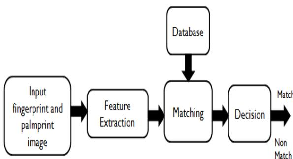
Fig.1. Block diagram of palmprint and fingerprint identification system.
