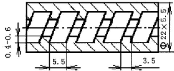
Figure 2. Schematic diagram of spirally internally ribbed tube
