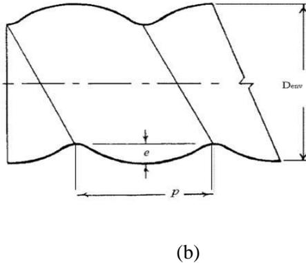
Figure 1. Tube's geometry (a) helical coil parameters (b) wall corrugation profile
