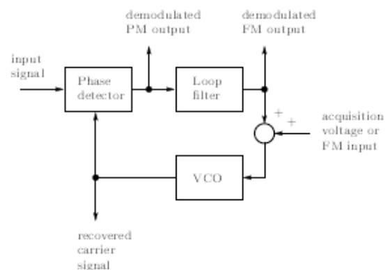
Figure 1: Block diagram Of Phase Locked Loop
