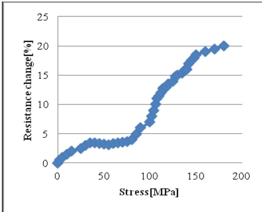
Fig.6. Typical Electrical response of the PVA-CNT fibers at 90° direction.
