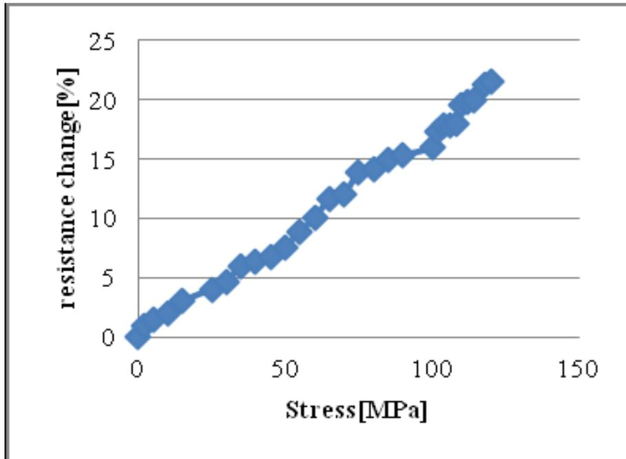
Fig.5. Typical Electrical response of the PVA-CNT fibers at 45° direction
