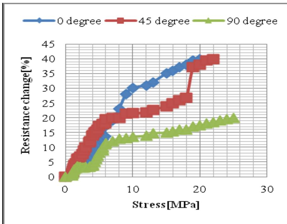
Fig.7. Comparison between the electrical responses of the corresponding direction of the PVA-CNT fibers sensor.
