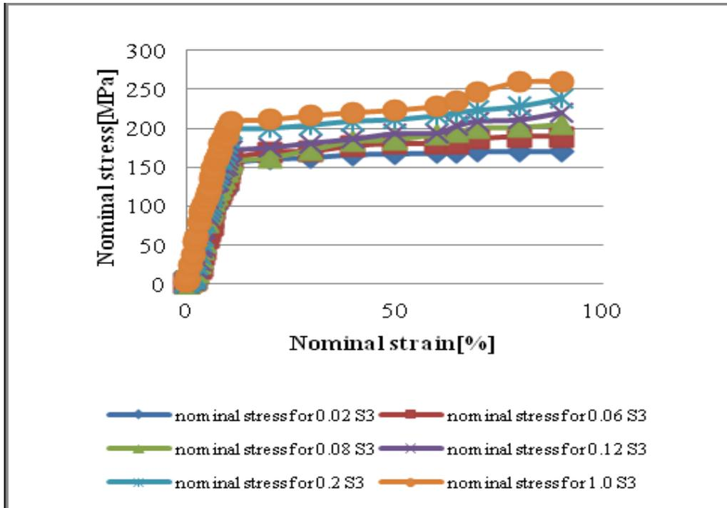
Fig.3. Typical mechanical response of the PVA-CNT fibers at 90° direction with different solvent weight ratio
