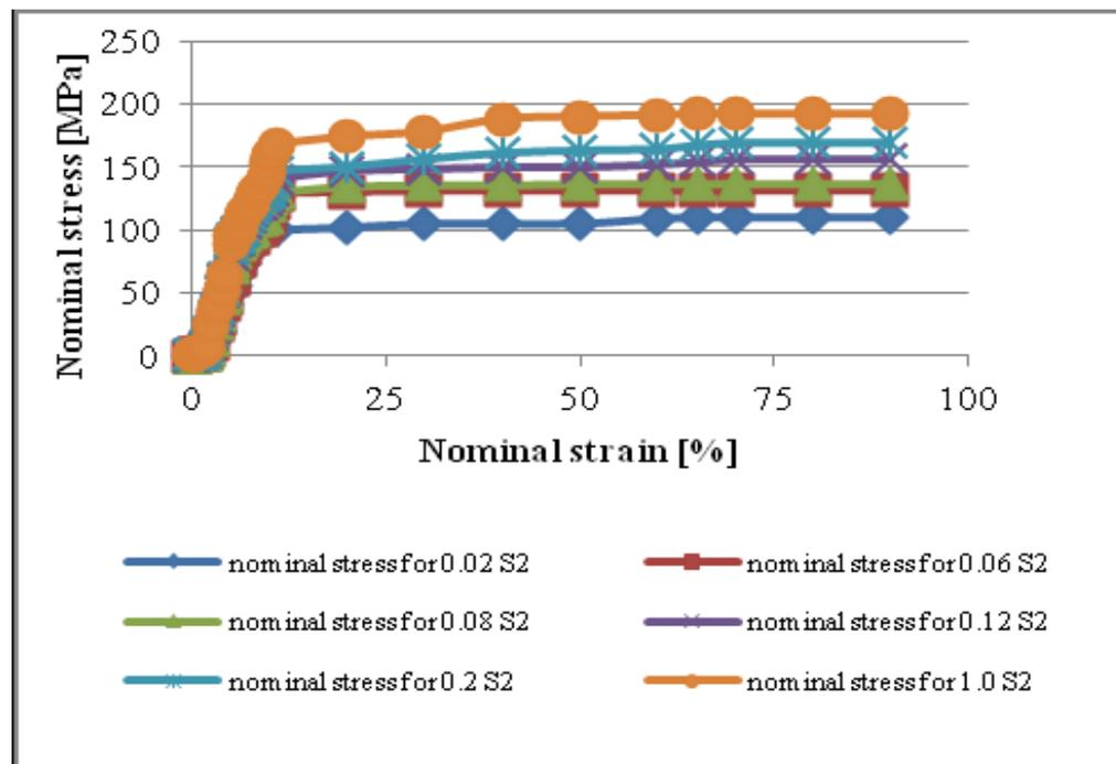
Fig.2. Typical mechanical response of the PVA-CNT fibers at 45° direction with different solvent weight ratio
