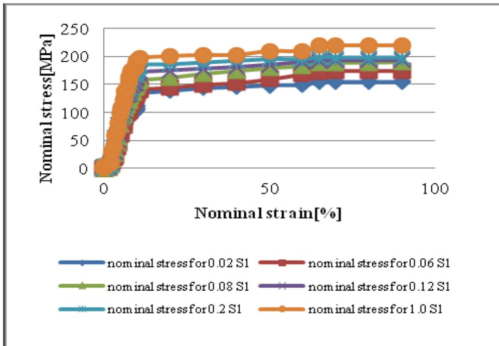
Fig.1. Typical mechanical response of the PVA-CNT fibers at 0° direction with different solvent weight ratio
