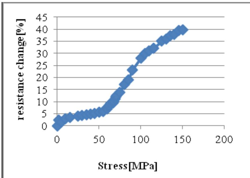
Fig.4. Typical Electrical response of the PVA-CNT fibers at 0° direction
