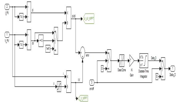
Fig.14 Incremental Conductance MPPT
