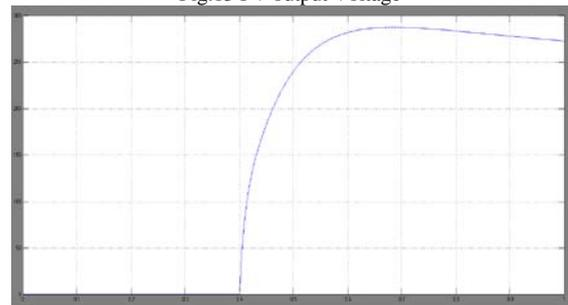
Fig.16 DC link Voltage with P&O MPPT
