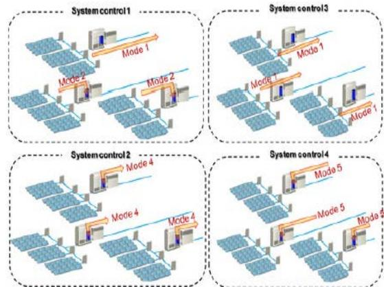
Fig.4 Example of different system operation modes of a RSC-based solar PV power plant
