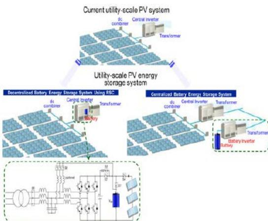
Fig.3 Utility-scale PV-energy storage systems with the RSC and the current state-of-the-art solution
