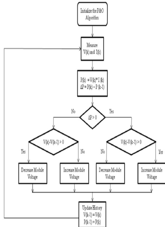
Fig.10 Perturb and Observe Algorithm
