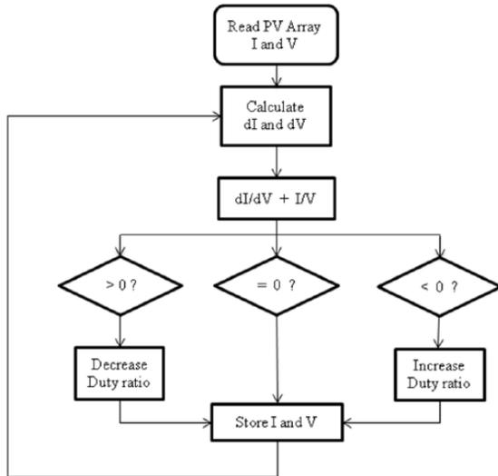
Fig.11 Incremental Conductance Algorithms
