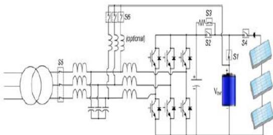
Fig.1 Schematic of the proposed RSC circuit
