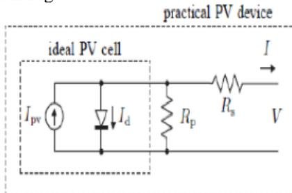
Fig.8 Equivalent circuit of ideal PV cell with  $R_p$  and  $R_s$ .
