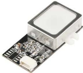
Fig. 1. Biometric Sensor GT511C3
