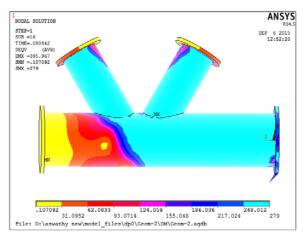
Fig.5.Von misses stress diagram of K3.
