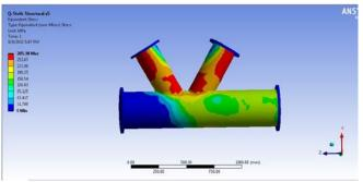
Fig.7.Von misses stress diagram of A2.
