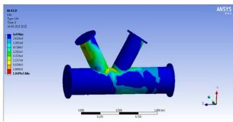
Fig.10. Life of specimen A1 at 2000 kN.
