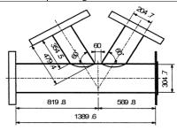
Fig. 1 Size of specimen.
