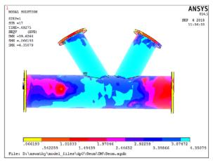
Fig.3.Von misses stress diagram of K1.
