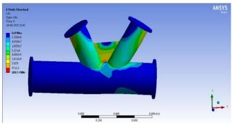
Fig.11. Life of specimen A2 at 2000 kN.
