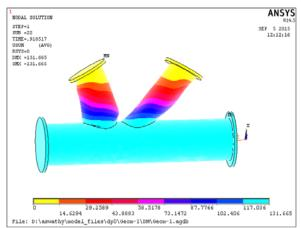
Fig.4.Von misses stress diagram of K2.
