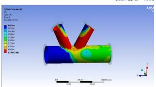
Fig.13. Life of specimen A3 at 3400 kN.
