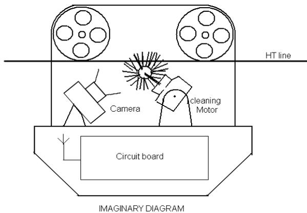
Fig. 3.1 Block diagram of inspection robot.
