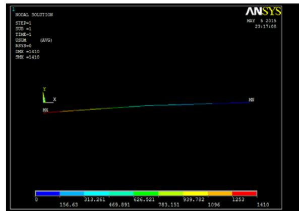
The maximum displacement in this case is found to be 1409.1mm
