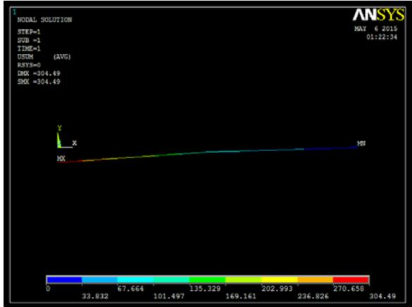
The maximum displacement in this case is found to be 304.49mm
