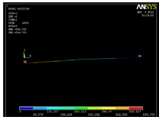
The maximum displacement in this case is found to be 594.71mm
