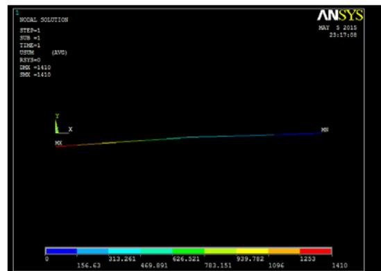
The maximum displacement in this case is found to 1409.7mm
