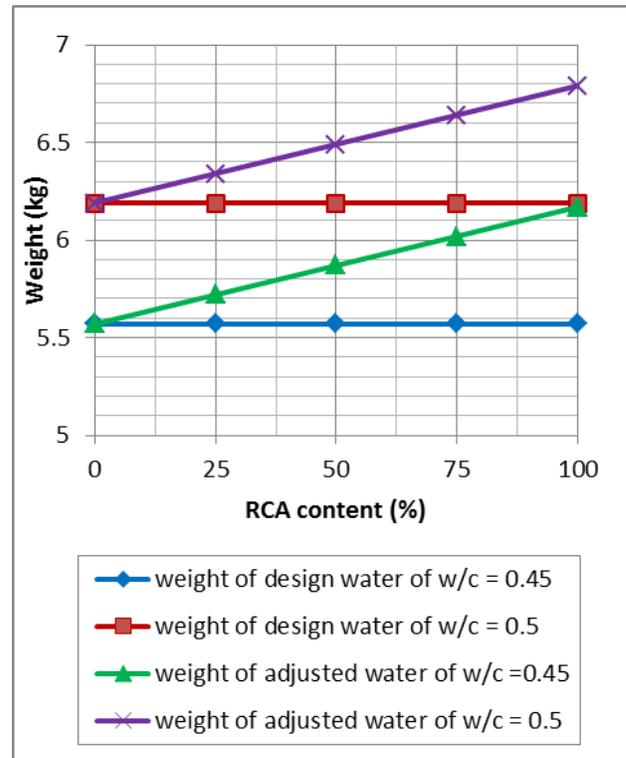
Fig. 2 Water used per 150 mm cube versus corresponding RCA content
