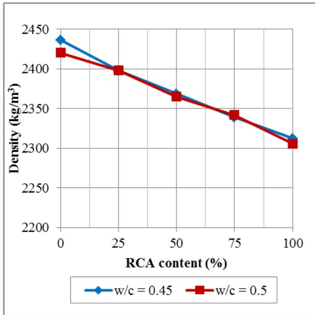
Fig. 7 Average densities of concrete cubes vs. RCA content
