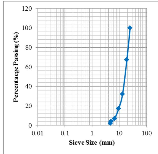
Fig. 1 Particle size distribution of RCA sample
