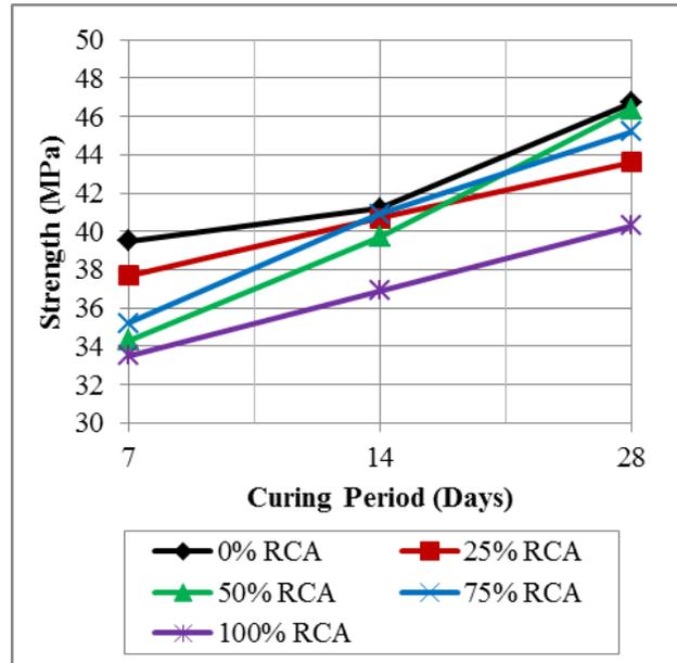
Fig. 4 Compressive strength of concrete cubes at w/c ratio of 0.45
