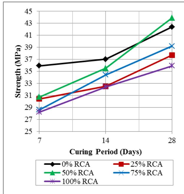
Fig. 5 Compressive strength of concrete cubes at w/c ratio of 0.5
