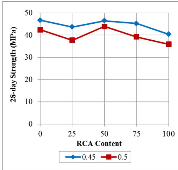
Fig. 6 Variation of compressive strength with RCA % replacement
