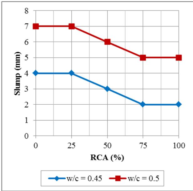
Fig. 3 RCA contents and corresponding slumps for both w/c ratios
