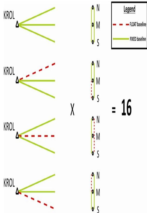
Fig. 6. Diagram of possible baselines in the unfailing rapid static approach.
