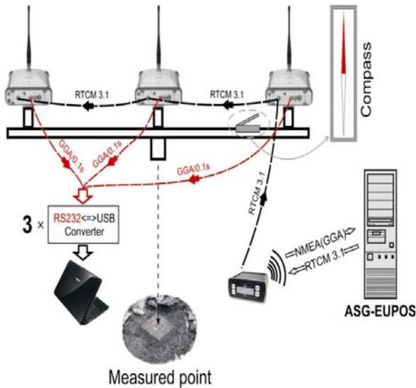
Fig.2. Hardware setup of the PS/GLONASS unit.
