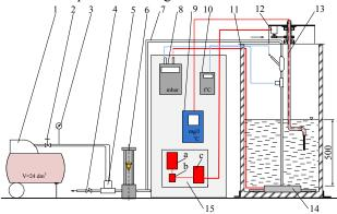
Fig. 10 Sketch of the experimental plant for researches regarding water oxygenation
