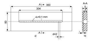
Fig. 1 The FBG perforated plate a) plan view; b) cross section.
