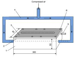
Fig. 2 Fine air bubble generator
