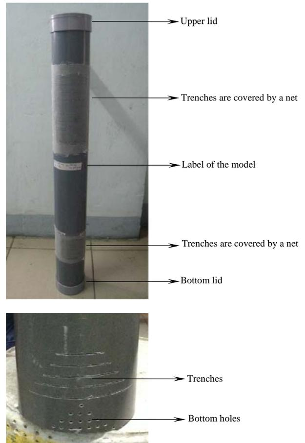
Fig. 3 Detail of the experimental model.
