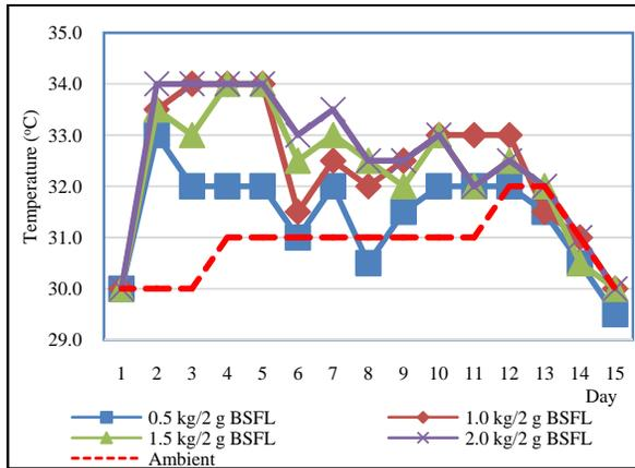
Fig. 5 Variation of temperature in the models.
