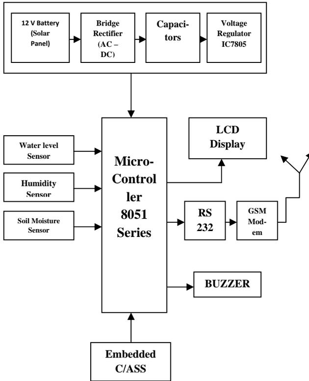
**Fig. 1 Architecture of Solar Panel Based Automatic Plant Irrigation System**
