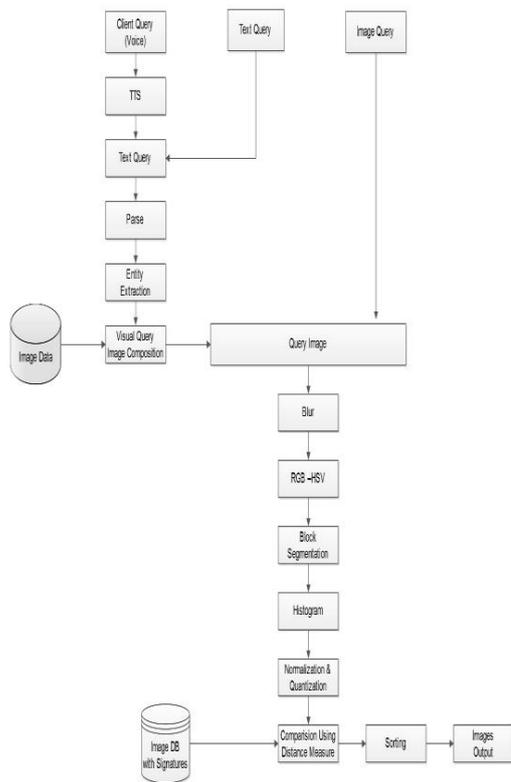
**Fig 1. The Architecture of multimodal image retrieval system**
