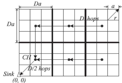
Fig. 2 The sensor field is partitioned into small grids with size  $a \times a$ . All nodes in a cluster-square of the size  $Da \times Da$  form a cluster, where the cluster head (CH) is located at the center.
