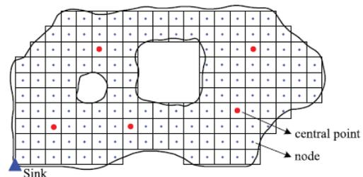
Fig. 1 An example of calculating the central points of cluster-areas: an irregular sensor field is roughly divided into small grids, and a virtual node is placed at the center of each grid. Five nodes are chosen as the approximate central points
