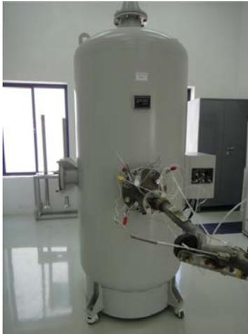
Fig. 8 Blower Tank – Experimental apparatus for setting engine conditions
