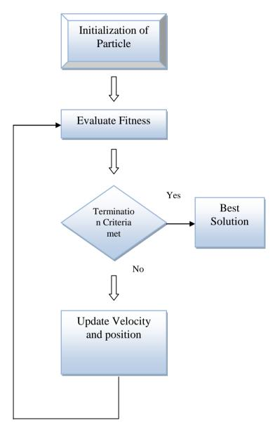
Figure 2 Flow Diagram of PSO Algorithm
