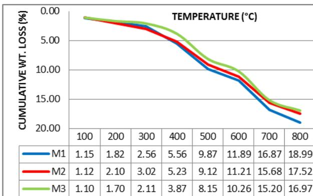
Fig.4 Thermal analysis of designed composites in air atmosphere, Heat rises@10°C/min
