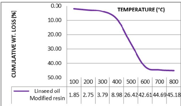
Fig.2 Thermal analysis of **Linseed oil Modified resin** in air atmosphere, Heat rises@10°C/min
