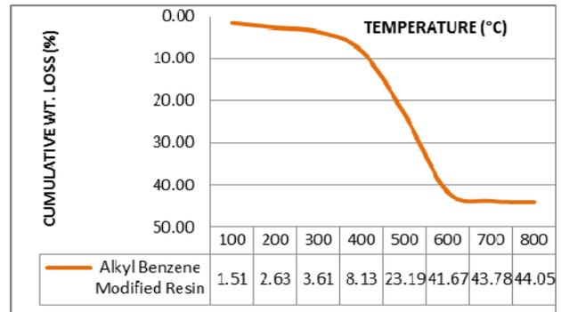
Fig.3 Thermal analysis of **Alkyl benzene modified resin** in air atmosphere, Heat rises@10°C/min
