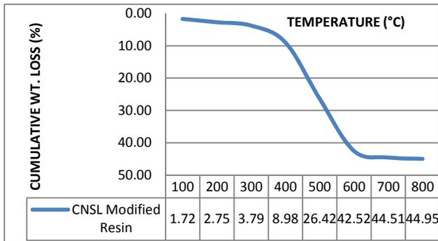
Fig.1 Thermal analysis of **CNSL Modified resin** in air atmosphere, Heat rises@10°C/min
