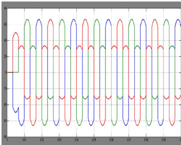
Fig.4 Three phase output voltage of 3-phase PWM drive
