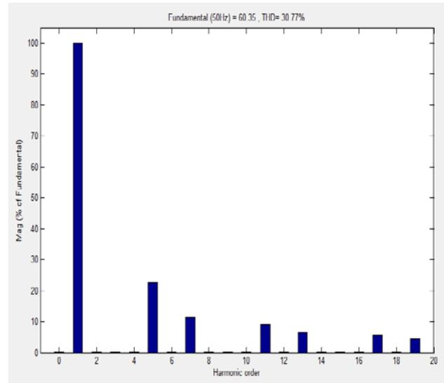
Fig.5 Harmonic Bar graph of 3-phase PWM drive
