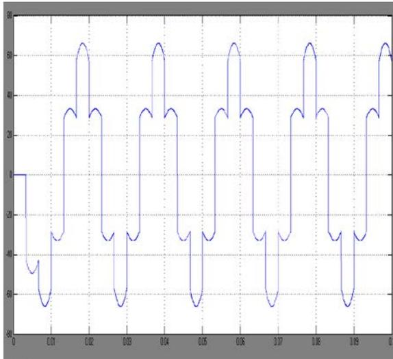
Fig.3 Single phase output voltage of 3-phase PWM drive
