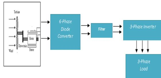
Fig.1 Block diagram of 3-phase PWM inverter drive with 6-phase generator
