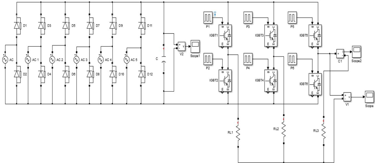
Fig.2 Circuit diagram of 6-phase converter with 3-phase PWM inverter drive
