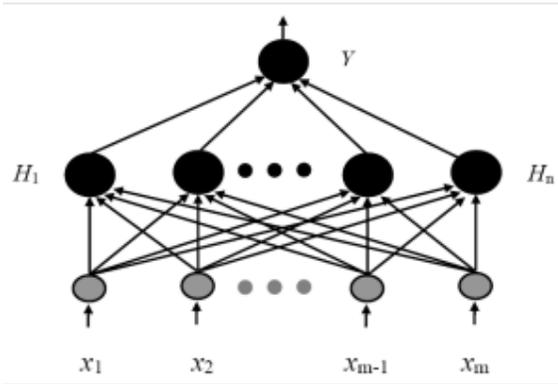
Fig. 3. A three-layered feed-forward NN model.
