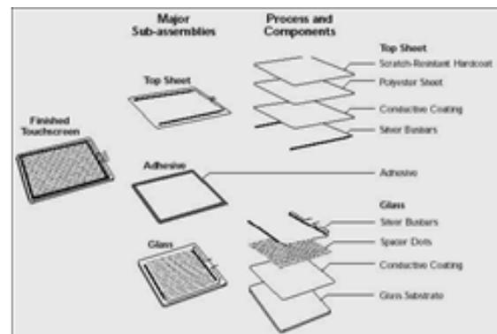
Fig. 1 The structure of resistive touch panel.
