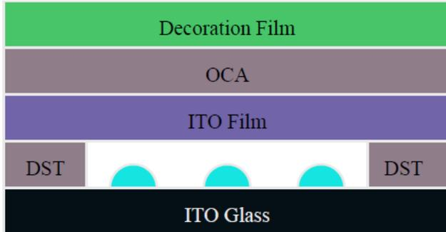
Fig. 2 The simple illustration of touch panel.
