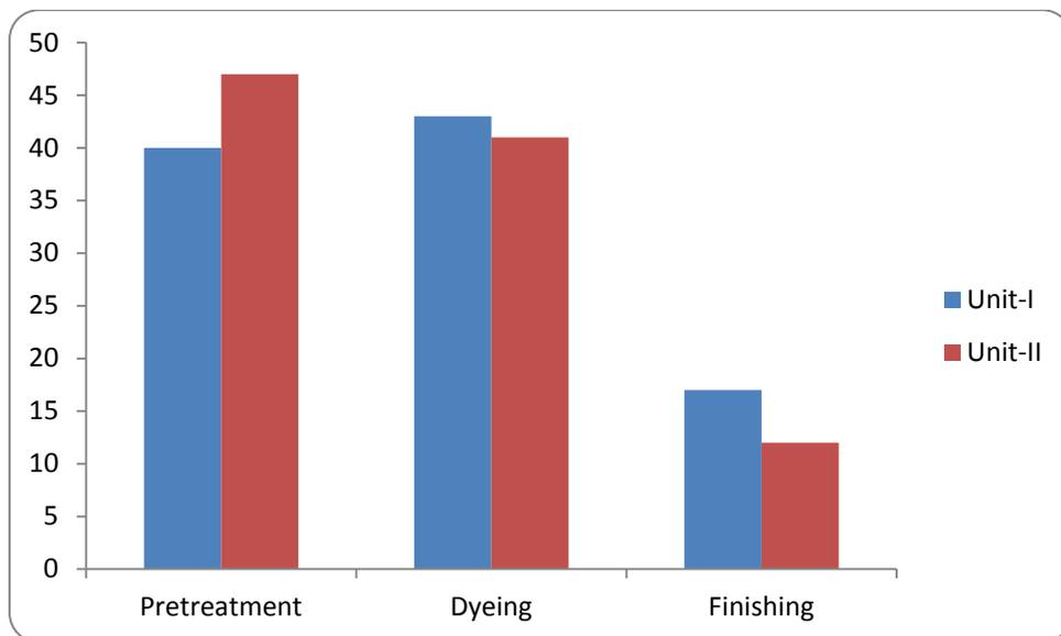
Figure-3.4 Processwise Percent Wastewater Generation in Unit-I & II
