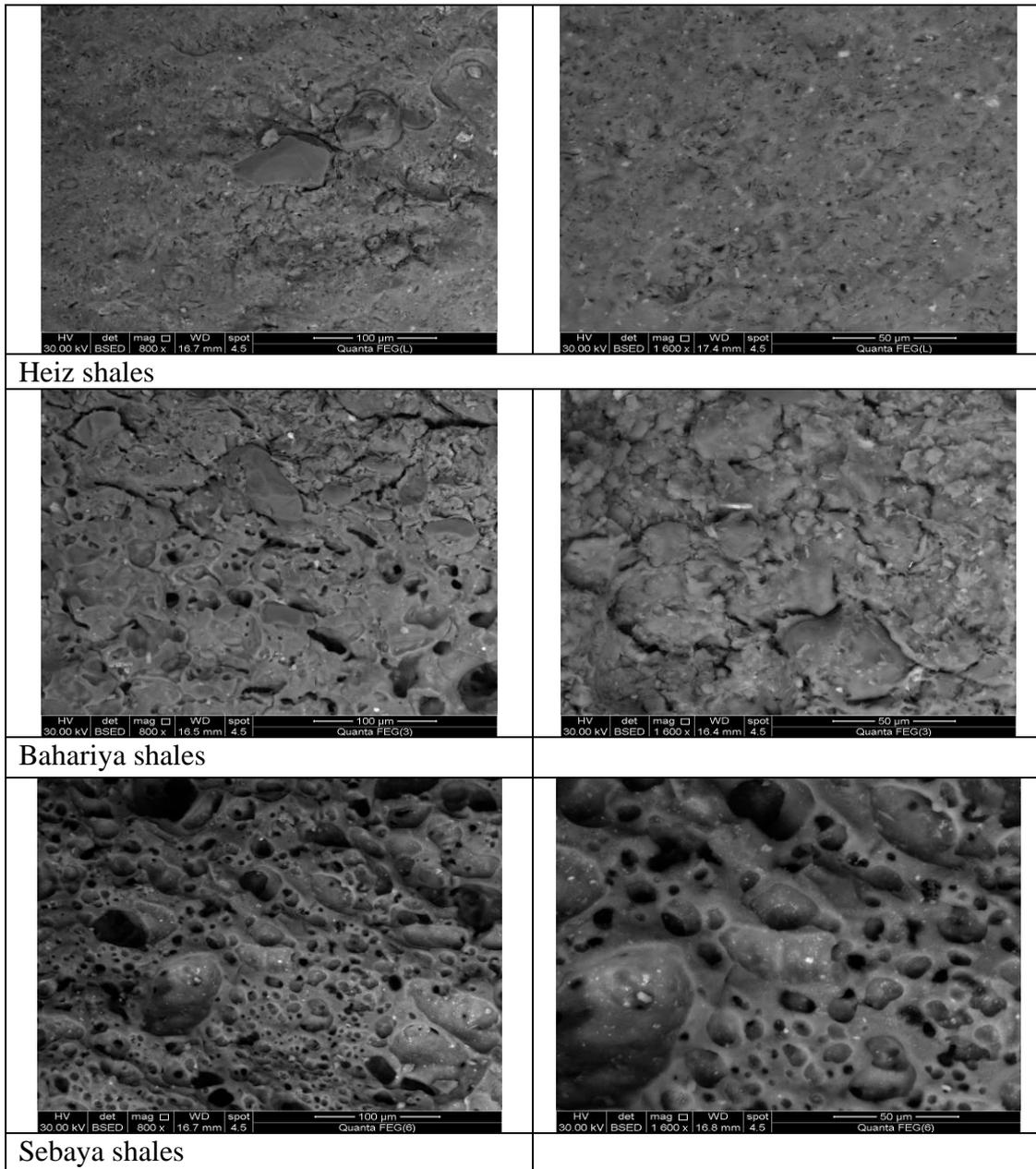
Fig.4. Close up view of SEM photomicrograph showing some shale samples fired at 1200°C.
