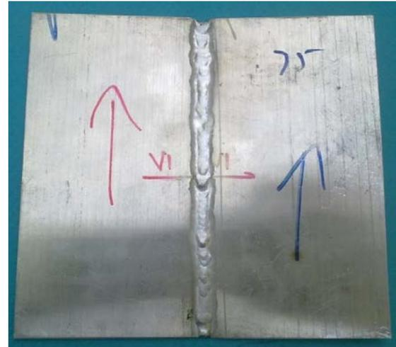
Fig. 1 The TIG Welded Aluminum TWB
