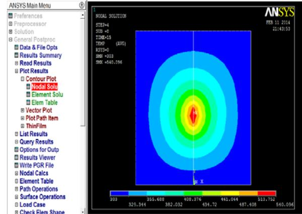
**Fig. 4. Simulation result of TWB at t=15 sec**
