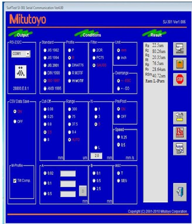
Figure 6: Profilometer value for pattern without coating
