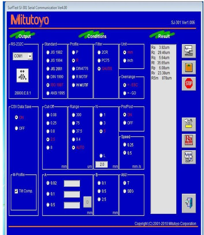
Figure 3: Profilometer value for graphite coated pattern
