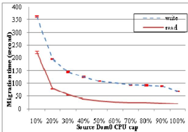
**Figure 5.** Migration time for Memory-intensive VM with Different CPU allocation to DomU on the source host
